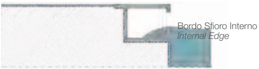
SFIORO INTERNO 1 DECREASED WATER LEVEL 1
