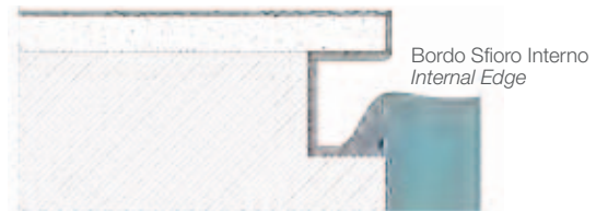
SFIORO INTERNO 2 DECREASED WATER LEVEL 2
